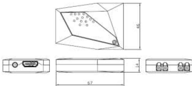
Note: The transmitter, HDFX-150-T and the receiver, HDFX-150-R have the same mechanical dimensions
